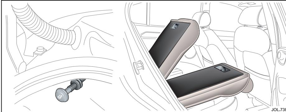
When returning the seat back to the upright position ensure that the seat belts are routed correctly and are not trapped by the seat back. Press the seat back firmly and check that it is locked securely into place.
