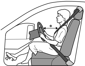
Correct: Belted and 254 mm (10 inches) or more away
