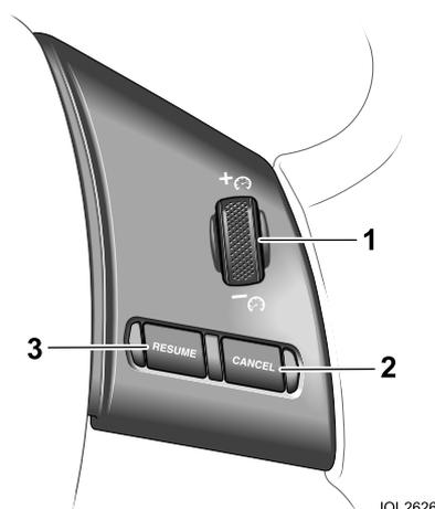
The cruise (speed) control system (where fitted) can be used by the driver to maintain a selected vehicle speed above 40 km/h (25 mph) without the driver having to use the accelerator.
