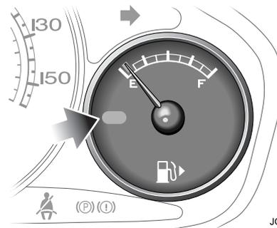
An amber lozenge in the fuel gauge illuminates when the remaining fuel has fallen to approximately 8 litres (1.75 gallons) including the reserve.
