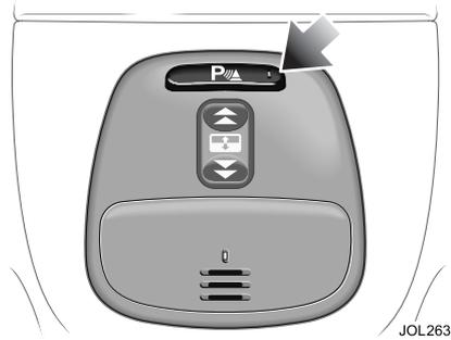
When both front and rear parking assist are fitted, a switch is located in the overhead console.
