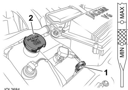
Remove the dipstick (1) and wipe clean with a non-fluffy cloth. Replace fully, then withdraw the dipstick. If the oil level is above the minimum mark on the dipstick then no additional oil is required.
