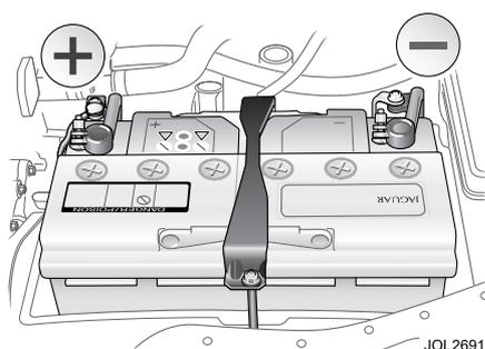
Open the bonnet and unclip the battery box cover. Remove the positive terminal cover.
