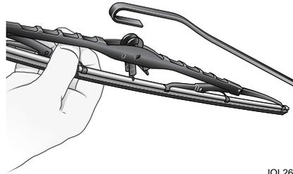
Move the wiper arm away from the windscreen, squeeze the retaining clip and withdraw the wiper blade from the arm. After fitting the new blade, check that it is held firmly in position. Reposition the wiper arm and blade onto the screen.
