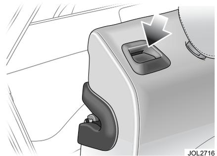
There is a red indicator to the rear of each release catch, which is only visible when the seat is unlatched.
