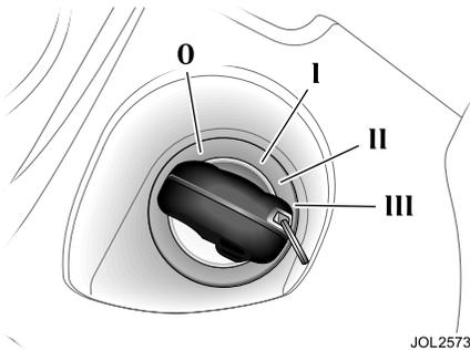
The ignition switch, on the right-hand side of the steering column, has four key positions:
