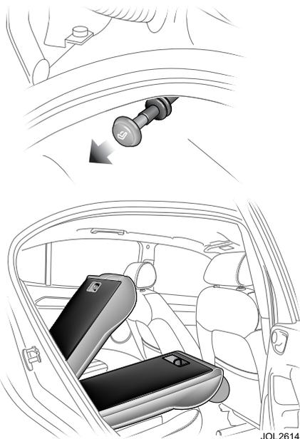
**Saloon:** Release handles for each seat back are in the luggage compartment under the parcel shelf. Pull the handle to release the seat back.
