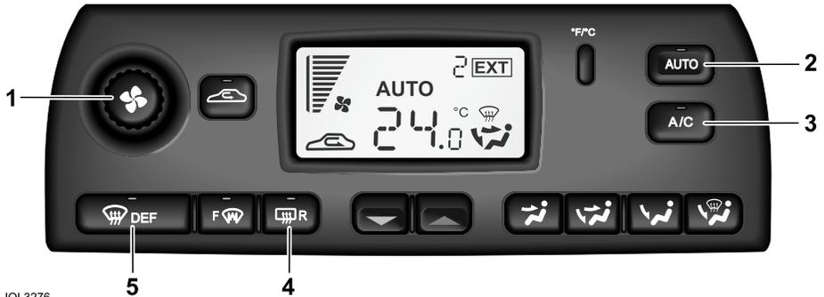
1. Push for system ON/OFF, rotate for manual blower speed.
