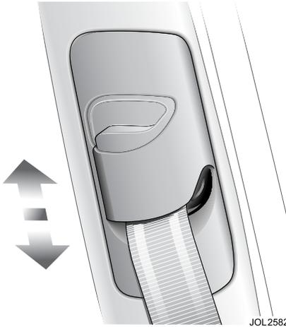
**To operate:** Press the locking button and slide the anchorage point to the required position to ensure comfort and safety. Release the button and check that the anchorage point is locked.
