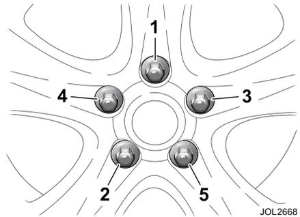
Fit the spare wheel and loosely secure with the wheel nuts.
