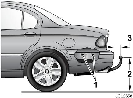
The rear longitudinal members are factory pre-marked (1) for drilling for tow-bar mountings. There are three mounting points on each side.
