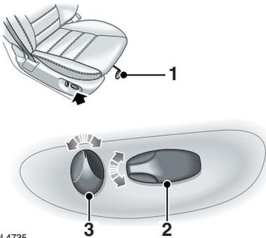
1. Seat fore/aft lever. Lift and slide to position.
