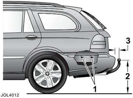
The rear longitudinal members are factory pre-marked (1) for drilling the tow-bar mountings. There are three mounting points on each side.
