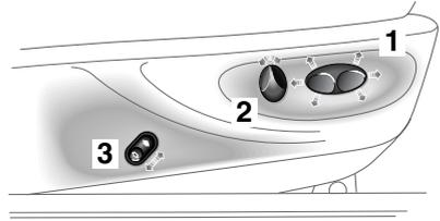
1. Seat position switch. Controls fore/aft position and front and rear cushion height.
