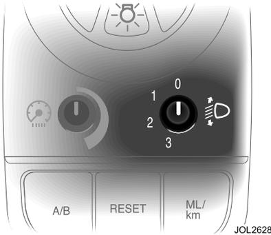
The headlight levelling switch operates when the headlights are switched ON. Push and release the knob to extend it for ease of operation. Push the knob again to place it in the stowed position.
