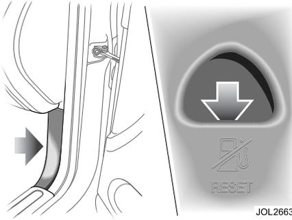
In the event of an accident, an inertia switch will trip, isolating the fuel supply. Once the switch has tripped it must be reset before attempting to restart the engine.
