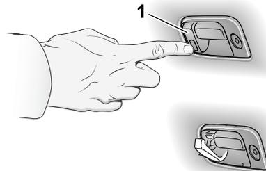
A hook for holding light-weight items such as a handbag, purse or small shopping bag is fitted beside the glove compartment lid release catch. Press the lower part of the hook (1) to lower the hook. Fold the hook back into the lid after use.
