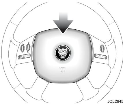
The dual tone horn is operated by pressing the centre pad on the steering wheel.
