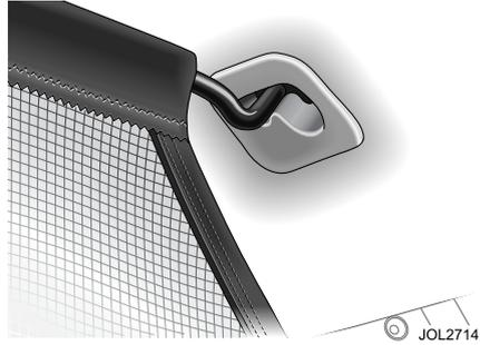
A luggage load net is fitted to some luggage cover housings. This can reduce the risk of luggage being thrown forward in the event of an accident, or under heavy braking. The load net can be retracted into the housing when not required.
