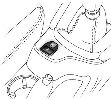
DSC uses traction control and anti-lock braking systems to maximise the vehicle's handling performance and help prevent wheelspin.
