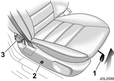
1. Seat fore/aft lever. Lift and slide to position.
