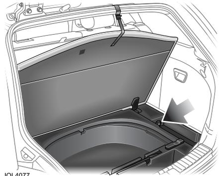
A 12-volt accessory socket is provided in the underfloor storage tray. The socket must only be used to power accessories that are temporarily connected to the vehicle.
