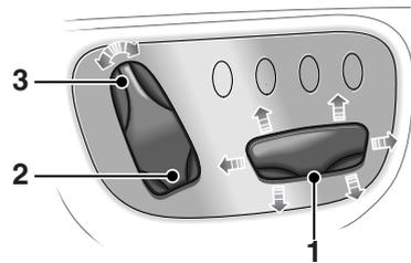
1. Seat position switch. Controls fore/aft position and front and rear cushion height.
