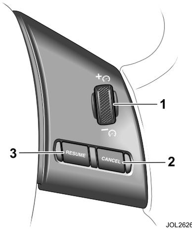
The cruise (speed) control system (where fitted) can be used by the driver to maintain a selected vehicle speed above 28 km/h (18 mph) for 2.5- and 3.0-litre vehicles, and 40 km/h (25 mph) for 2.0-litre petrol and diesel vehicles, without the driver having to use the accelerator.
