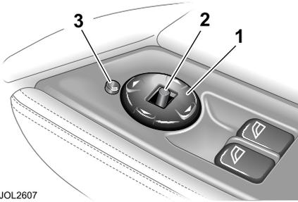
Both door mirrors are adjusted from the driver's door switchpack. The four-way adjustment button (1) moves the mirrors to the required position. The selector switch (2) selects the mirror to be moved, left for the left-hand side mirror and right for the right-hand side mirror. When the selector switch is in the centre position, adjustment to either mirror is inhibited.
