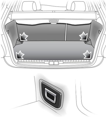
Four metal loops are positioned in the luggage compartment for attaching straps to secure loads and prevent them from sliding over the luggage floor.
