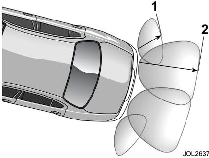
When reverse gear is selected and the ignition is on, rear parking assist provides an audible warning when reversing the vehicle if obstacles are detected within range of the rear of the vehicle, as shown in the illustration above.
