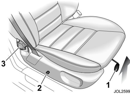
**Forward and rearward:** Each front seat can be adjusted forward and rearward by lifting the locking bar (1), situated below the front of the seat cushion and sliding the seat to the required position. After releasing the locking bar, slight additional seat movement may be necessary to engage the locking mechanism.
