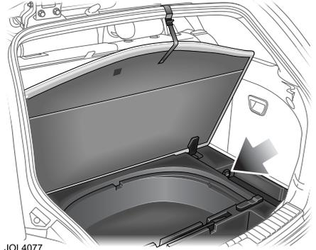
There is an underfloor storage tray located below the floor panel. Lift the floor panel (there is a handle on the rear edge) to access the storage tray.
