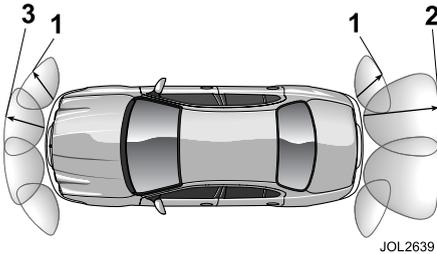
The front parking assist provides an audible warning when driving forwards if objects are detected within range of the front of the vehicle, as shown in the illustration above.
