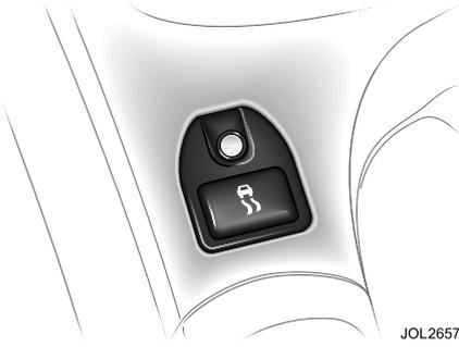
Dynamic stability control is operational whenever the engine is running, unless it has been switched off. If the system is operating, the warning light in the instrument cluster will flash.
