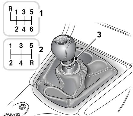
A diagram of the gearshift pattern, either six speed (**1**) or five speed (**2**) is set in the top of the lever knob.
