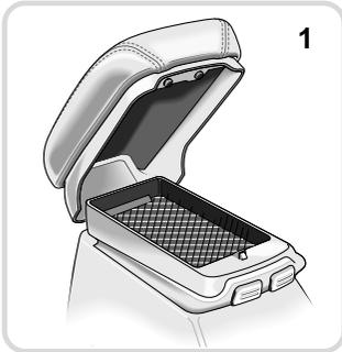
The sliding armrest is hinged at the rear and has two release buttons located on the front of the armrest.
