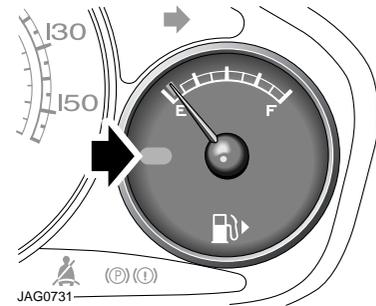
An amber indicator on the fuel gauge (arrowed) illuminates when the remaining fuel has fallen to approximately 8 litres (1.75 gallons) including the reserve.
