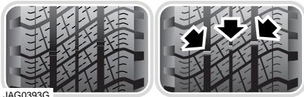
It should be noted that the properties of many tyres alter progressively with wear. In particular the wet grip and aquaplaning resistance are gradually but substantially reduced. Extra care and speed restriction should therefore be exercised on wet roads as the effective tread depth diminishes.
