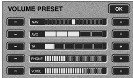
After touching the **Volume** button, the screen displays the buttons for adjustment of volume associated with the navigation system, JaguarVoice, telephone, Traffic Announcements (TA) and Automatic Volume Control (AVC). Adjustment of AVC varies the rate at which volume is increased or decreased relative to vehicle speed.
